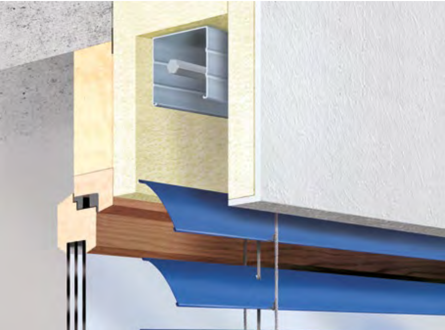
Horizontal section for crank drive
